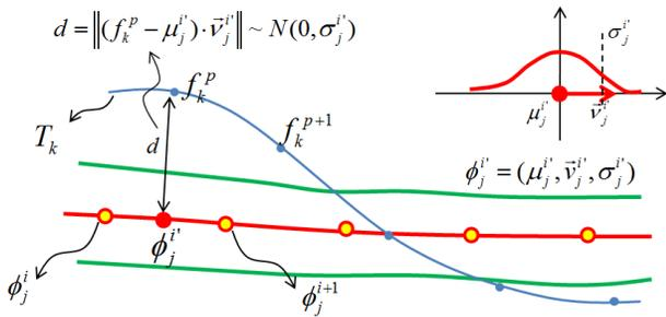
Fig. 4. An illustration of distance between a route centroid and a trajectory frame
