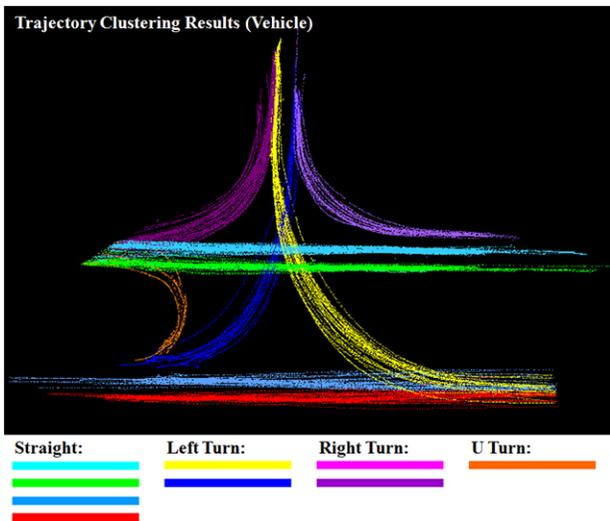
Fig. 6. The clustering result of vehicle trajectories
